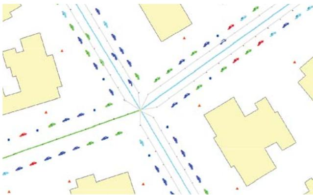
**FIGURE 1** To represent a two-way traffic street, the centerline is duplicated, and each copy is employed for representing one direction. Parking places are built parallel to the street, with a distance of 4 m between the places.
