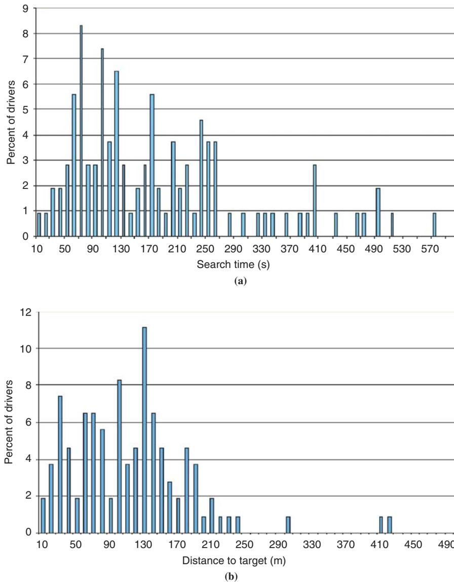
FIGURE 4 Typical model outputs (driver's view): (a) distribution of search time and (b) distribution of distance between parking place and final destination.
